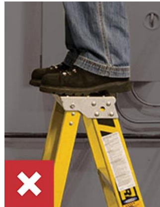
WRONG DON'T stand above the second step from the top of a stepladder or the fourth rung from the top of an extension ladder.
